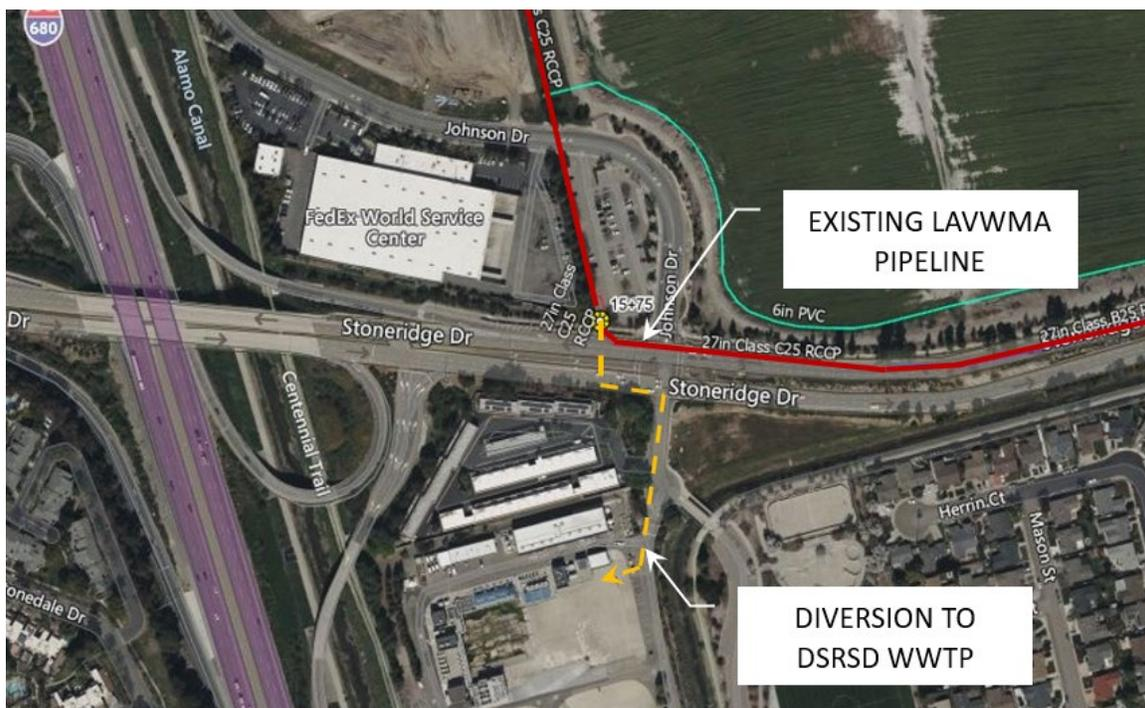
Figure 3-2. Overview of potential diversion of Livermore’s secondary effluent to DERWA
