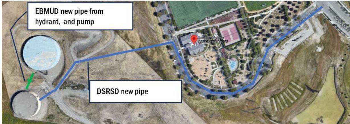
**Figure 3-6. Overview of infrastructure required for longer-term addition of potable water at Reservoir R100**
